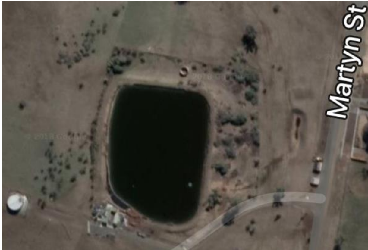
Figure 1 – Aerial view of the Taralga Water Supply Treatment Facility featuring Off River Storage Pond, Water Treatment Component Cluster, Circular Treated Water Storage Reservoir and disused buildings located on Martyn Street road reserve.
