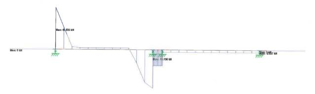
Figure 50: Shear Force diagram for a strip of the deck
