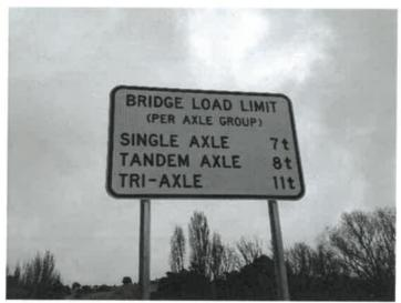
Figure 1: Current bridge loading limits
